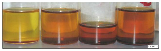
A1: Change in pure biodiesel in storage at 50 °C. Oxidised fuel components give biodiesel a dark colour.
